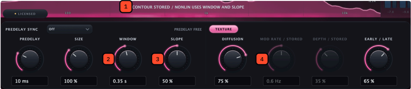
FIG. 3 In NONLIN, DECAY becomes WINDOW, BLOOM becomes SLOPE, and controls NONLIN does not use read STORED. 1 Display note. The contour is stored; NONLIN uses WINDOW and SLOPE. 2 WINDOW. The length of the gate or reverse window. 3 SLOPE. Reverse, through gated, to decaying. 4 STORED. A control this space does not use keeps its value. VITRICAUDIO.COM 8 / 24
