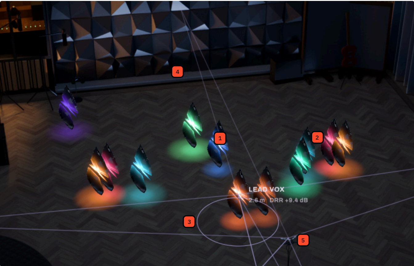
FIG. 2 The stage in STAGE view: every track stands in the room as a lit glass shard over its pool of light; the selected Lead Vox shows its label, its ring and its reflection paths to the listener. 1 The selected track. Lit in its color. 2 Its label. Name, distance and DRR. 3 Ring and pool. The light on the floor. 4 Every other track. Lit by its own level. 5 The listener. The array at the seat. VITRICAUDIO.COM 7 / 38
