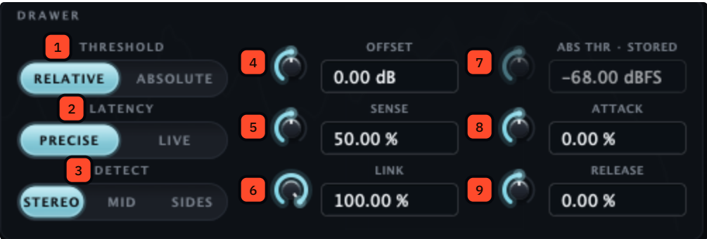
FIG. 6 The drawer at its defaults: RELATIVE threshold, PRECISE latency, STEREO detection.
